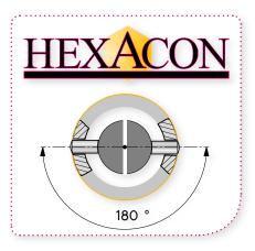
PMK precision meas. heads • Functional description PMK measuring heads are used for the reliable, rapid precision measurement of diameters and form errors in holes of a wide variety of types.
